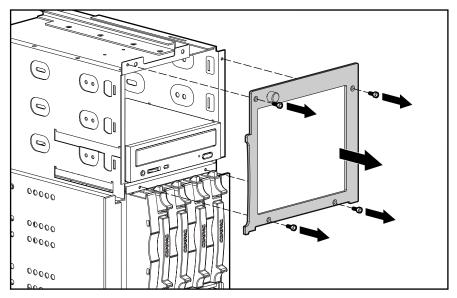
Figure 2-21. Removing the removable media panel
